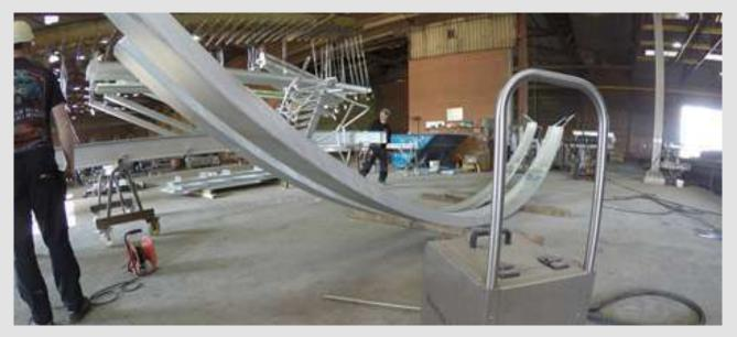
Removal of spots with zinc ashes is done in seconds without any damaged to the surface. We supply mobile units that can be used at multiple locations, where standard compressed air plugs are located.
