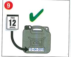
TwinOxide solution is ready for use for approx. 30 days — write the date of preparation on the label of the container.
