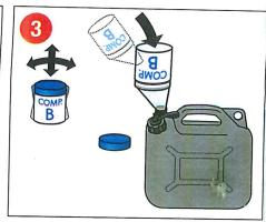
First, shake the jars of powder, and add component B to the container with water.
